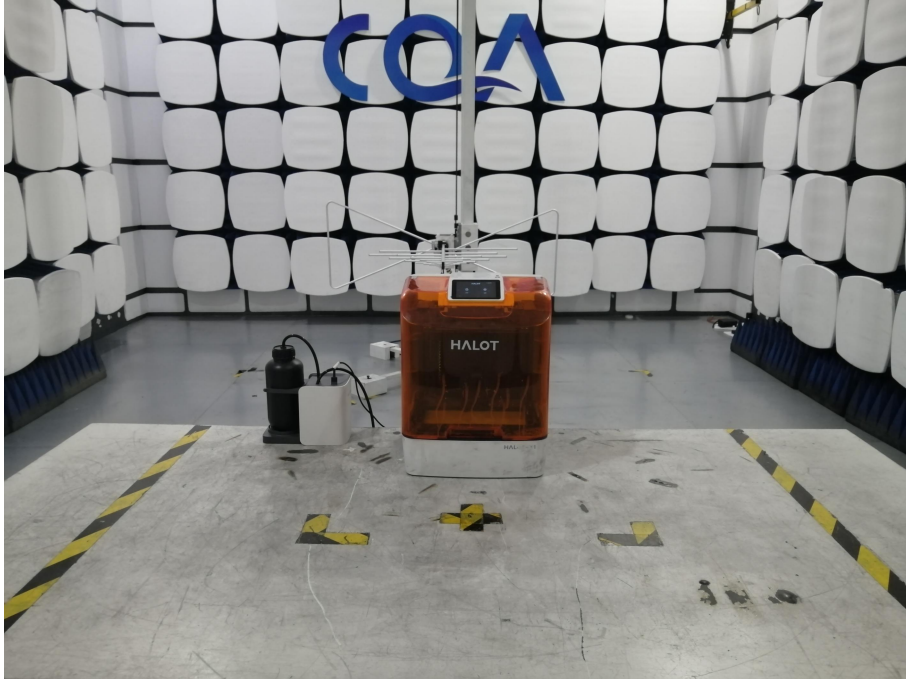
Radiated emission Test Setup (30MHz~1GHz)
